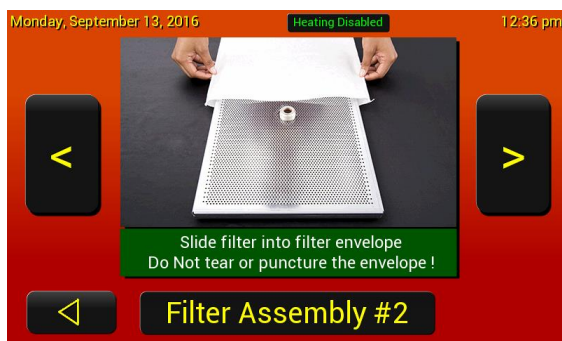
Preparing a fryer filter for use ...
