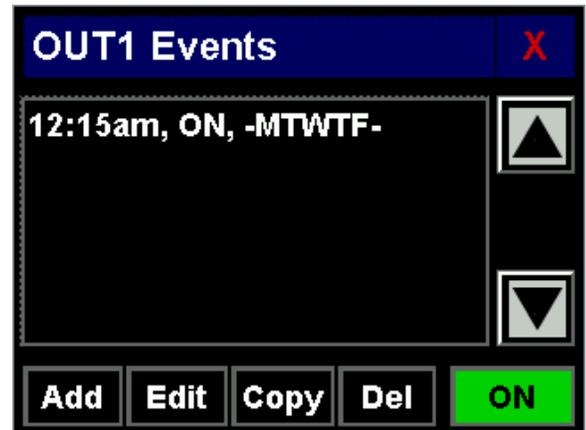
The **[ON]** button indicates that this output schedule is active. Touching this button disables the schedule, the button turns black and the text changes to **[OFF]**. Touching the button again re-enables the schedule, the button turns green and the text changes to **[ON]**.
