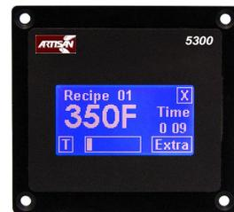
**Electrical Specifications:** Operating Voltage: 115V or 230V AC, RTD Inputs - 100 Ohm 385 DIN curve, Output Relays - 10A resistive, DC Outputs - 12V DC at 25mA maximum, Beeper - 103dB at 10cm.
