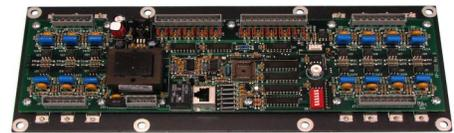
**Iced Tea Dispenser Controller** - This product was designed for the Pepsi-Lipton Partnership for a series of sweetened and unsweetened iced tea dispensers. It provides thermostatic control of a hot water heater, time of day lockout of the dispenser requiring regular sterilization the system, Hall Effect sensors for dispensing handle detection, and variable output speed control of the primary product pump.
