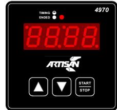
**Electrical Specifications:** Operating Voltage - 12V DC, 24V AC, 115V AC, and 230V AC; Timing Accuracy -  $\pm 0.5\%$ ; LED display - 0.56" high high intensity red LED, Output Relay - 20A resistive or inductive; Operating Temperature - 0°V to 70°C; Mounting - 2.62" square opening, bracket with single mounting nut.
